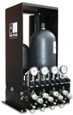
Shore Western manifolds have full flow 10 micron filtration for the main circuit, and where applicable, 3 micron full flow filtration for the servo valve pilot and hydrostatic bearing circuits. Fluid filtration protects components downstream from impurities in the hydraulic oil.
