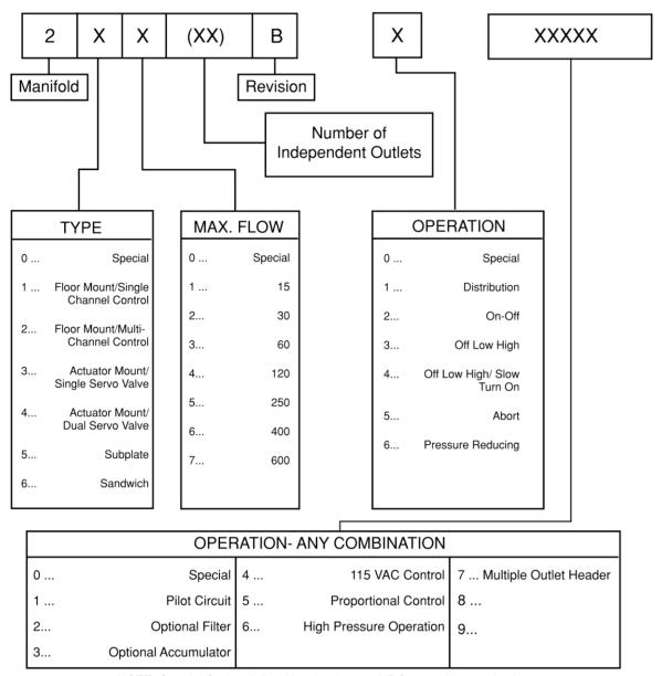
NOTE: Special Codes defined by drawing; 24 VDC control is standard
